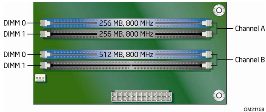
Figure 16. Dual Channel Memory Configuration with Three DIMMs
