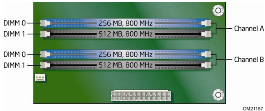
Figure 15. Dual Channel Memory Configuration with Four DIMMs
